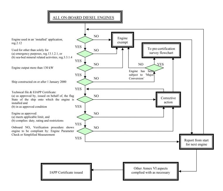
Figure 2 – Initial survey on board a ship
