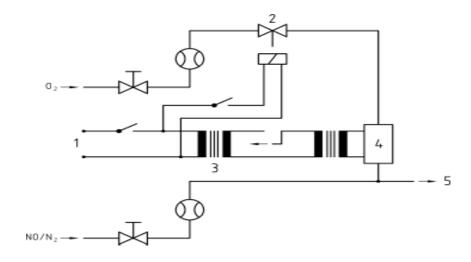
Figure 1 – Schematic representation of NO<sub>2</sub> converter efficiency device
